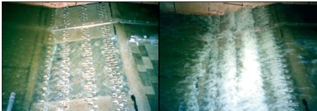
Fig. 5.21: Performance of roughness elements showing the degree of turbulence
