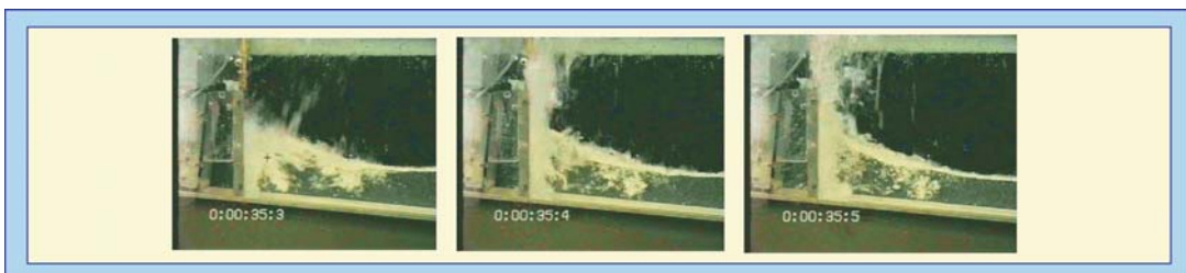
Fig. 7.5: A broken wave at a vertical wall, resulting in a broken wave overtopping condition
